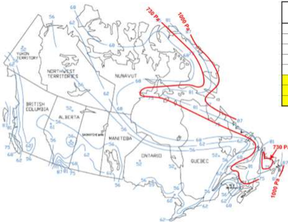
Map of wind speed (mph) contours in light blue, pressures (Pa) in red where greater than 720 Pa.
