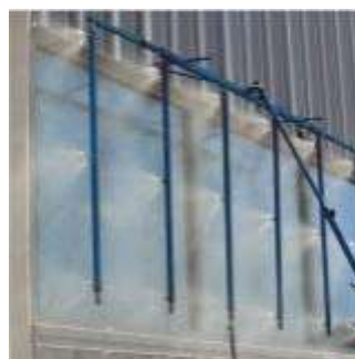
A window spray rack
