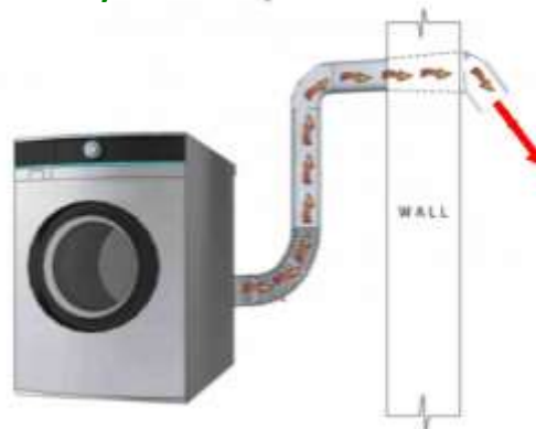
A laundry dryer exhausting directly through a wall to the outside
