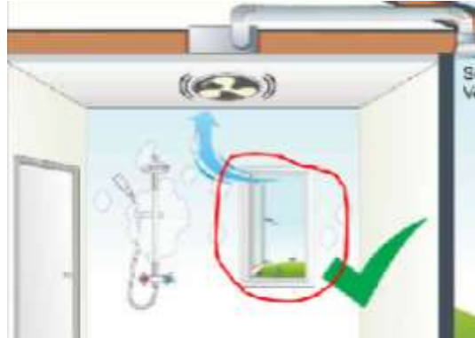
Air flowing into a bathroom with a steamy shower and the exhaust fan running
