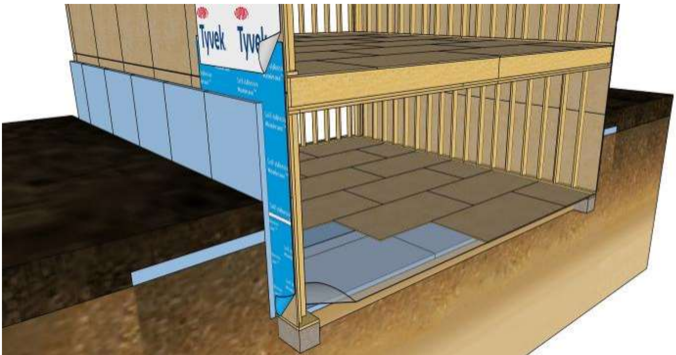
House with a wood-framed basement
